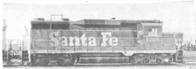
EMD / GP30 / 2250 hp / 4 axles B-B wheel arrangement SANTA FE 3200-3284 (1200-1284) / SP 5010-5017 / UP 700 series
