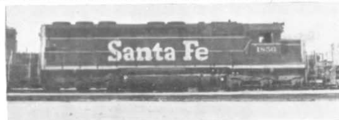
EMD / SD45 / 3600 hp / 6 axles C-C wheel arrangement SANTA FE 5500-5615 (1800-1889) / SP 8800-9155 / UP 3600 series
