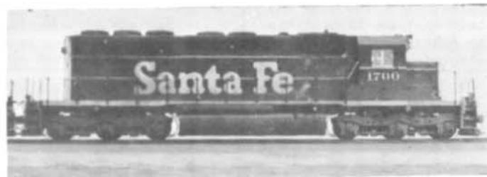
EMD / SD40 / 3000 hp / 6 axles C-C wheel arrangement SANTA FE 5000-5019 (1700-1719) / SP 8400-8478 / UP 3000 series
