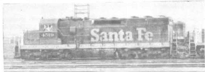
EMD / SD24 / 2400 / 6 axles C-C wheel arrangement SANTA FE 4500-4579 (900-979) / UP 400-429
